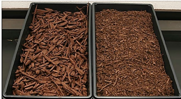
Impact Dark Brown colored at 3 #/yd on "bigs" (left) vs. "fines" (right)
