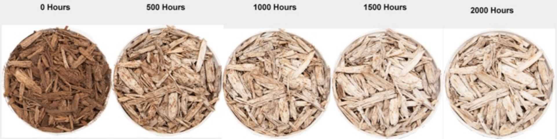
Figure 1 - Actual images of Screened Mixed Hardwood - (0 Hours thru 2000 Hours)
