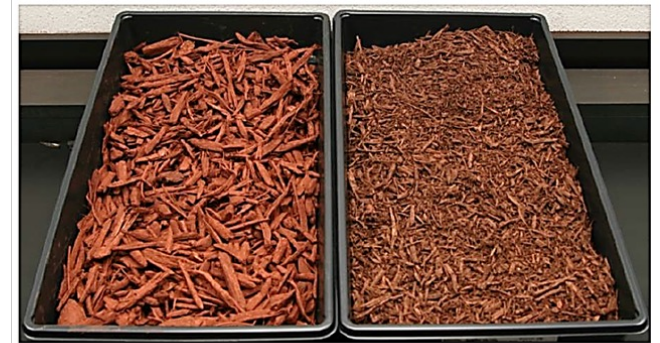
Impact Red colored at 3 #/yd on "bigs" (left) vs. "fines" (right)
